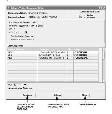
Figure 790-12. ATM Bundled VC Multicast Connection Status Window
